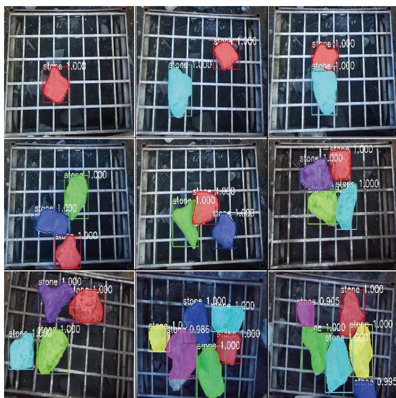
Fig. 8. The improved Mask RCNN ore identification and segmentation results
